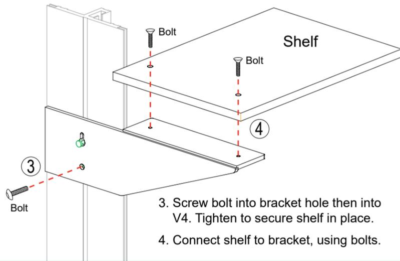
3. Screw bolt into bracket hole then into V4. Tighten to secure shelf in place.
