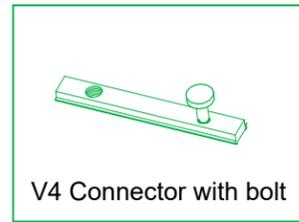
1. Slide V4, with bolt, into groove of vertical extrusion then tighten bolt to secure V4 at desired location.
