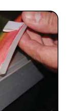
Insert narrow side of silicone welt into the channel at corner **1**, with fabric to the outside.
